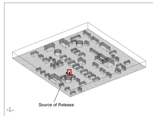
Figure 8. Computation Volume Model in COMSOL of Industrial Site and Source of Release
